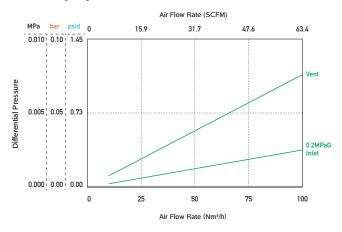
\*SCFM: Temperature 21.1°C (70°F), Humidity: 0% RH, Standard pressure (101.3kPa)
