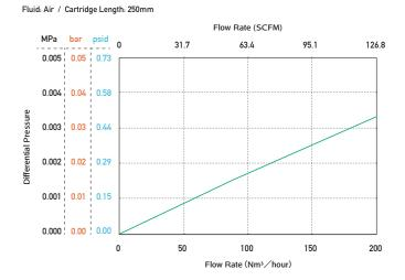
\*SCFM: Temperature 21.1  $^\circ C$  (70  $^\circ F$ ), Humidity: 0% RH, Standard pressure (101.3 kPa)
